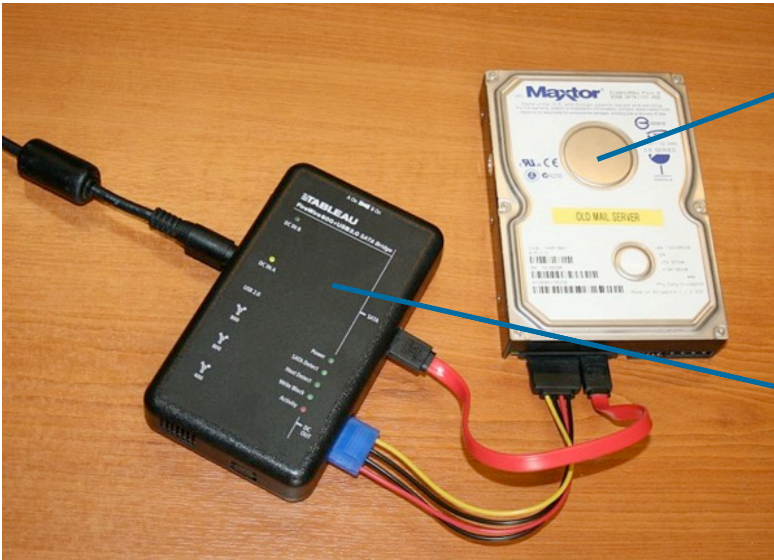
“Write Blocker” prevents accidental overwriting.
